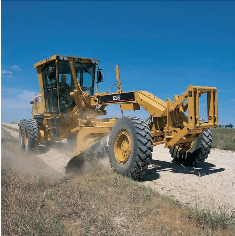
**Quiet Cab.** The resiliently mounted engine and transmission provide interior sound levels of 76dB(A) when measured with the doors and windows closed per ISO 6394. Lower interior noise levels improve operator working conditions.
