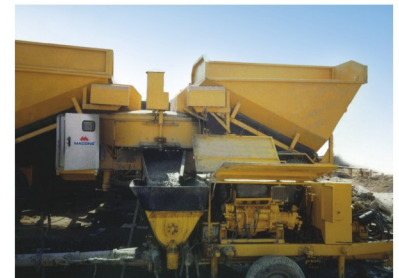
Mixed Concrete discharged directly in to the Concrete Pump
