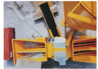
Top view showing four aggregate hoppers
