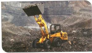
Hydrostatic drive with automotive control, 2 stages shiftable under load, single lever (Joystick) for drive and working hydraulics control.
