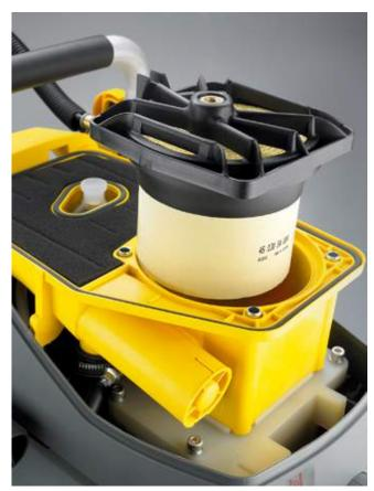
The pulled in air passes first through the cyclone filter where the majority of dirt particles are already removed. This is followed by the foam material prefilter. The pre-cleansed air only meets the main filter at the end of the process. This results in a manifold increase of the air filter's service life. In addition, there is only minimal loss of pressure. This ensures a consistently high engine performance.
